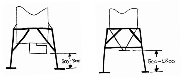
This means that the height for scraper bottoms can be between 300mm to 800mm (from ground to gear).
