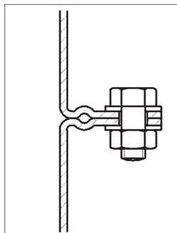
Fig. 1. Flange connection with beaded flanges.
