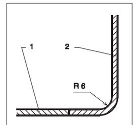
Fig. 5. Detail of inlet based on method 2.
