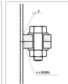
Fig. 2. Flange connection with welded flanges.
