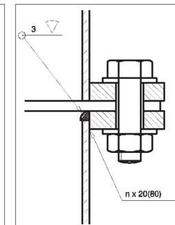
Fig. 3. Connection to the tube sheet method 2.
